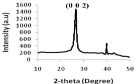
Fig.2: XRD Pattern of MWCNTs
