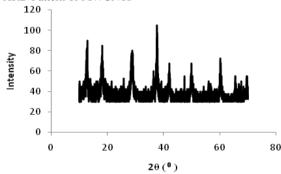
Fig.3: XRD pattern of 10 wt% MWCNTS/MnO2
